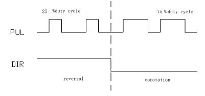
1. this control mode through the pulse duty cycle to control the speed, the effective duty cycle speed range is  $10\% \sim 90\%$ , the corresponding speed range is  $0 \sim (P06-40 \text{ setpoint}) *10$ . The recommended pulse frequency range is  $1K \sim 20K$ . The corresponding formula between duty cycle and target speed is as follows:
