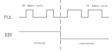
1.this control mode through the pulse duty cycle to control the torque, the effective duty cycle torque range is  $10\% \simeq 90\%$ , the corresponding torque range is  $0 \simeq (P06-43 \text{ setpoint}) *10$ . The recommended pulse frequency range is  $1K \simeq 20K$ . The corresponding formula between duty cycle and target torque is as follows:
